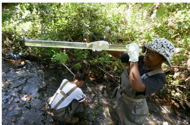
Cape Winelands Biosphere Reserve citizen scientists measuring the clarity of water using a turbidity tube.
